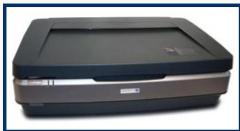
A highly sensitive flatbed scanner for most common nonfluorescent densitometric applications in the life sciences, especially electrophoresis evaluation. The scanner has a linearity above 3.4 OD, with 16-bit pixel depth, providing accurate quantitation and high sensitivity of very faint images without additional filters.
