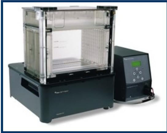
Ettan DALTwelve System can run simultaneously up to 12 large-format gels in 4 to 6h. The system streamlines performing second-dimension SDS-PAGE separations, increasing productivity while delivering high throughput, resolution, and reproducibility. When used in combination with 24 cm Immobiline™ DryStrip gels, Ettan DALTwelve maximizes the number of discrete, quantifiable protein spots obtainable per large-format gel.
