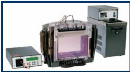
Ettan™ DALSix Electrophoresis Unit runs up to six large format (26×20cm) second-dimension polyacrylamide gels in just 4-5h. The gels accept first dimension 18- or 24-cm Immobiline DryStrip gels (IPG strips) from both Ettan IPGphor™ and Multiphor™ II isoelectric focusing systems. The system components include Ettan DALSix Electrophoresis Unit, Gel Caster and Gradient Maker, an EPS 601 Power Supply, and MultiTemp™ III Thermostatic
