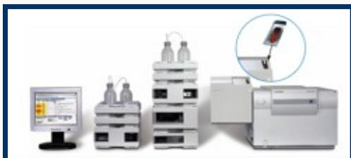
This mass spectrometer is constituted by a chip based nano-chromatography system, interfaced to an ESI source coupled to an Ion Trap analyser. The fragmentation power of ETD is integrated, providing a "softer" mode of fragmentation than classical CID, thus preserving protein labile modifications. ETD and collision induced dissociation (CID) modes of fragmentation from scan to scan help to pinpoint the
