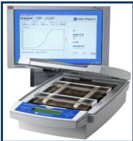
The Ettan™ IPGphor™ 3 IEF System is a fully integrated isoelectric focusing system optimized to deliver speed and reliability in the first dimension of 2-D electrophoresis. The instrument runs up to 12 IPG strips (7, 11, 13, 18, or 24 cm) simultaneously using Ettan IPGphor Manifold, Ettan IPGphor Manifold Light, or ceramic strip holders. Its lid design allows optimum running with light-sensitive protein samples, such as 2D-DIGE. The Ettan IPGphor 3 Control Software is also available.
